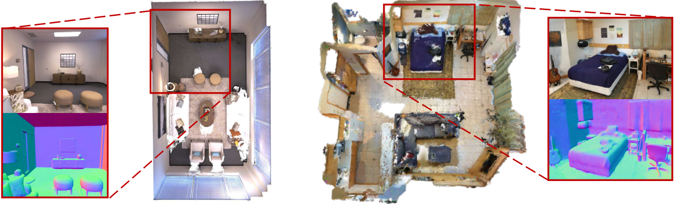
Fig. 1: Reconstruction results of 2DGS-SLAM on synthetic dataset Replica [74] and real-world dataset ScanNet [10]. We present the reconstructed 2D Gaussian splatting maps, along with RGB and normal renderings from zoomed-in local views. These results demonstrate that our method achieves both high-fidelity image rendering and precise geometric reconstruction.
