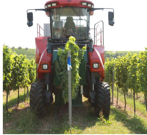
Figure 3: Field phenotyping platform called Phenoliner [10]. The Phenoliner is based on a grapevine harvester. The harvesting equipment is replaced by a calibrated stereo camera system. The camera system produces overlapping images of the plants covering approximately 1.2 m vertically of the wine row.
