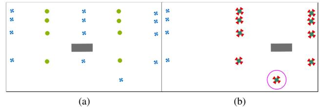
Fig. 7: An ambiguous situation is resolved over time. (a) The vehicle pose (gray) is undetermined as it could either be in the left or in the right side of the image. The correct map associations between map landmarks (blue) and observations (green) are unclear. (b) With an additional landmark detection over time (purple circle) the setting is correctly assessed such that all true map associations (red) are found.
