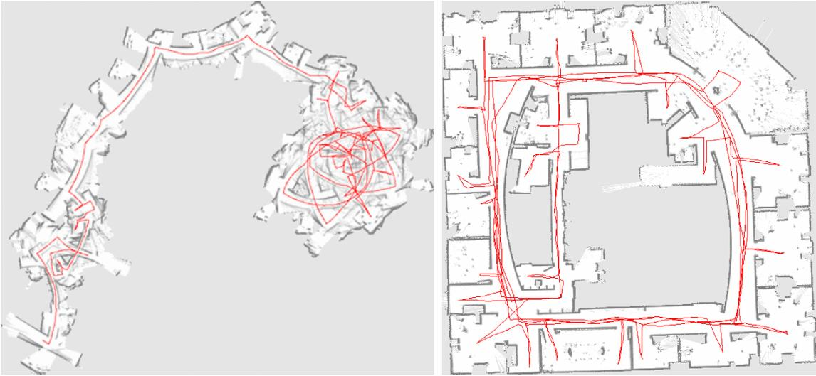
Figure 5: Occupancy grid map generated from laser range data and based on pure odometry. Image courtesy of Dirk Hähnel, University of Freiburg.
