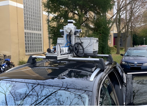
Figure 5. Sensor setup we used for recording data for the PANIC dataset. The setup includes four cameras, one GNSS/IMU device, and two 3D LiDARs. For further details, please refer to Vizzo et al. (2023).
