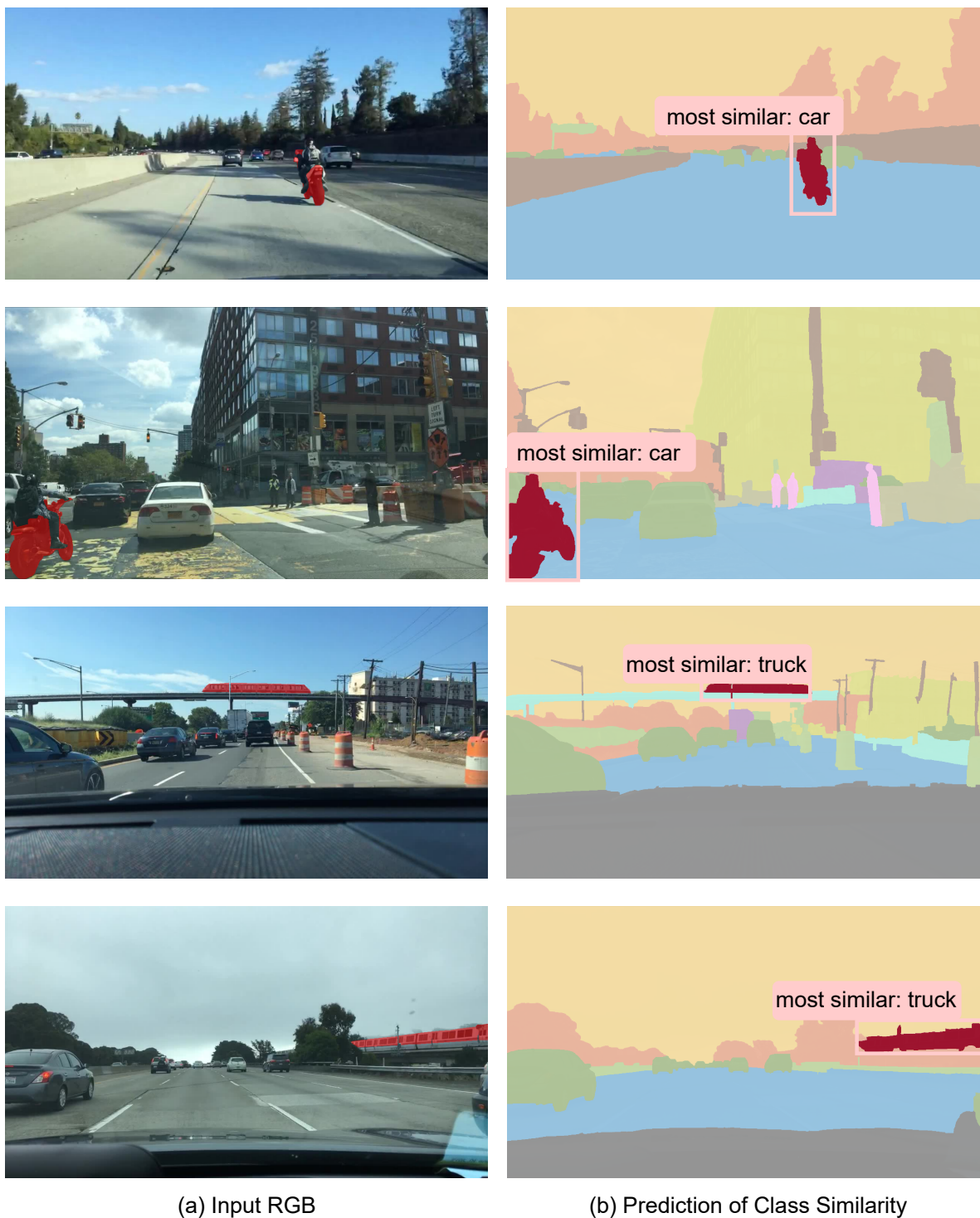
Figure 7. Class similarity results from the test set of BDDAnomaly. We show the input RGB overlayed with the ground truth unknown mask (a) and the prediction of our class similarity pipeline (b). In the open-world prediction, the unknown class is shown in red, and the overall semantic segmentation is shown in transparency.
