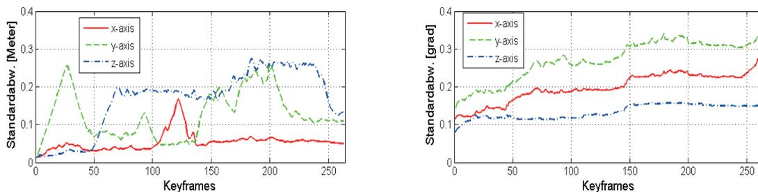
**Figure 4: The estimated standard deviations of the obtained position (left) and rotation (right) regarding to the first keyframe. The estimated inner uncertainty is given for 273 keyframes.**
