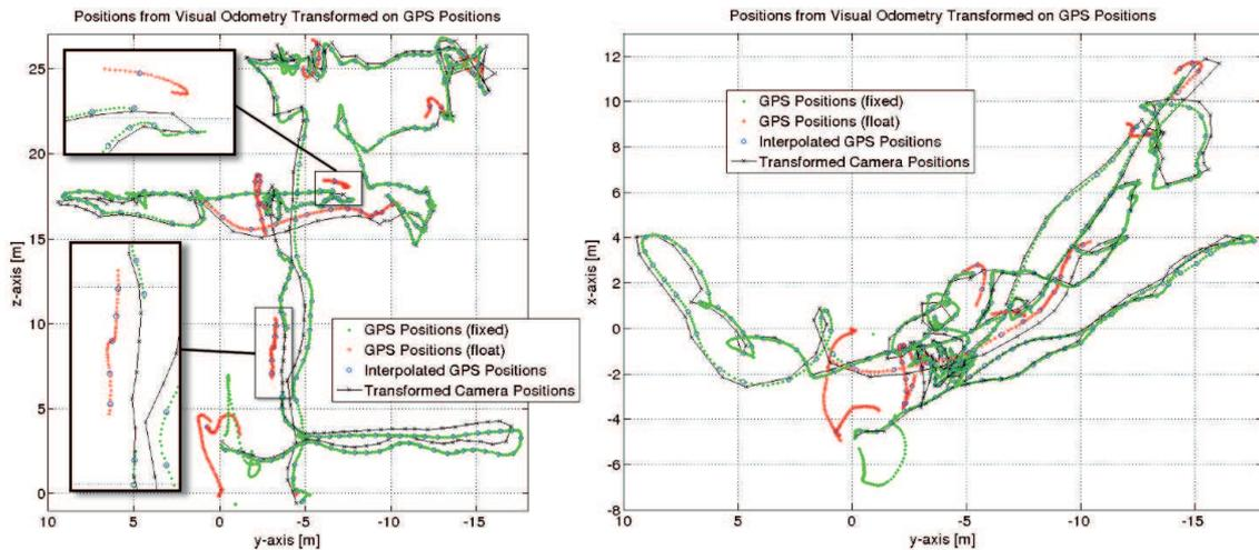
**Figure 3: The onboard processed trajectories of the georeferencing unit and transformed incremental bundle adjustment. Left: Lateral view on the trajectories in the yz-plane, note the capability of the visual odometry to bridge float solutions of the georeferencing unit. Right: Top view on the trajectories in the xy-plane.**
