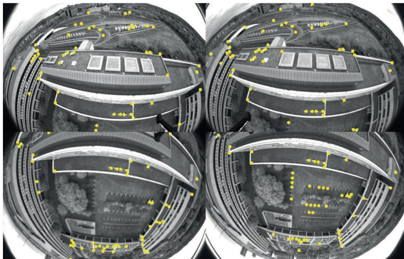
**Figure 2:** A frame set consisting of four images taken with the four fisheye cameras. Each image contains 50 interest points, which are tracked using the KLT tracker from the OpenCV library.
