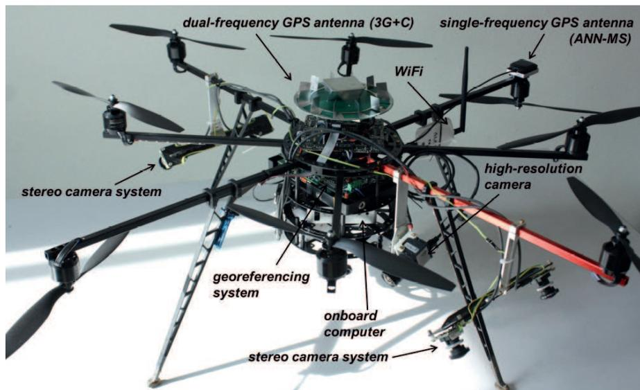
Figure 1: Sensor setup of the UAV (picture taken from Klingbeil, L. et al., 2014).
