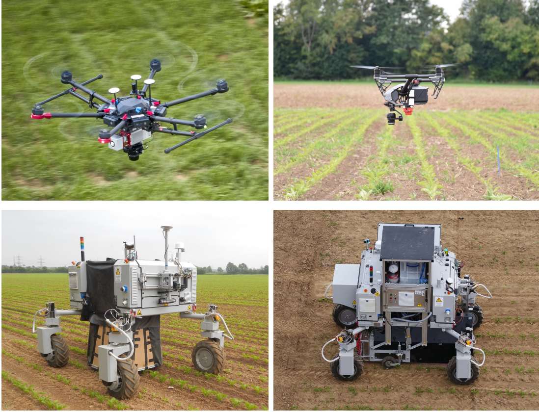
Figure 1.1: Examples of robotic platforms used in agriculture. The first row shows UAVs equipped with different cameras flying over the crop fields. The second row shows UGVs deployed in the fields. In the image on the left, we can see how the area below the robot is isolated to control the light condition of the captured images.
