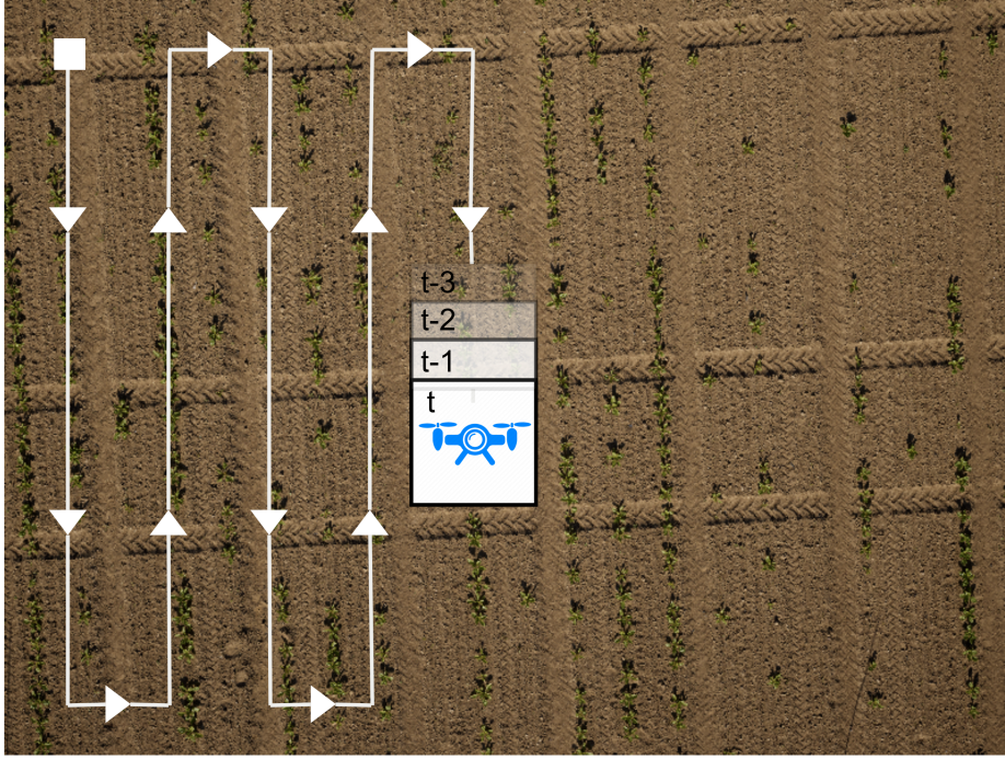
Figure 5.2: Example of a typical UAV mission. The coverage path along which we fuse semantic image labels is depicted in white, the square is the initial pose, and the arrows indicate the direction of movement. The images can overlap, but it is not required. This path ensures efficient coverage of the crop field and is commonly adopted in aerial data collection missions.
