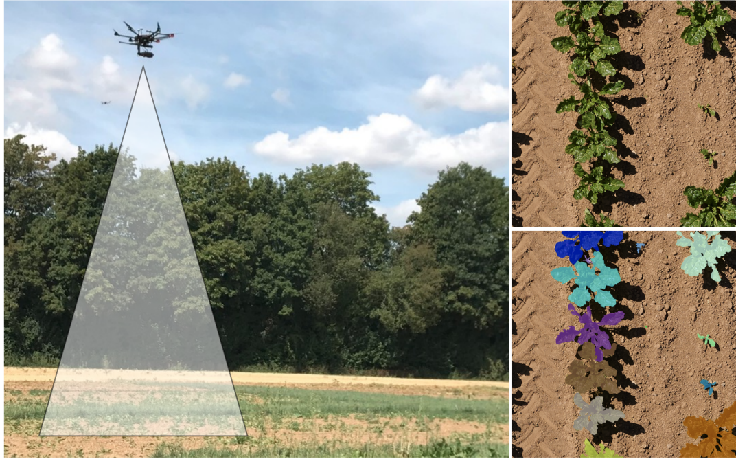
Figure 6.1: Robotic UAV systems equipped with RGB cameras, such as the drone shown in the left image, can capture images of agricultural fields for monitoring purposes. On the right we can see one exemplary image and the desired result for the plant instance segmentation task, where we assign a unique identifier to each plant. In the image, different identifiers correspond to different colors.
