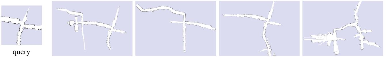
Figure 2: Example of the submap retrieval using FabMAP2. The left image shows the query map, the other ones the best four matches from the database.
