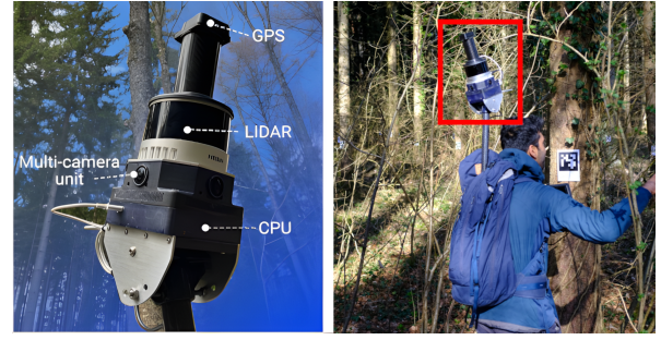
Fig. 3: For the DigiForests dataset, we recorded data with a (left) backpack-carried sensor payload in (right) challenging forest environments with the sensor payload highlighted in red (right).
