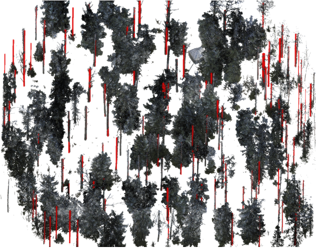
Fig. 5: Qualitative results of our cylinder fitting approach. Cylinders are shown in red. The point cloud has been cropped along its height to allow clearer visualization.
