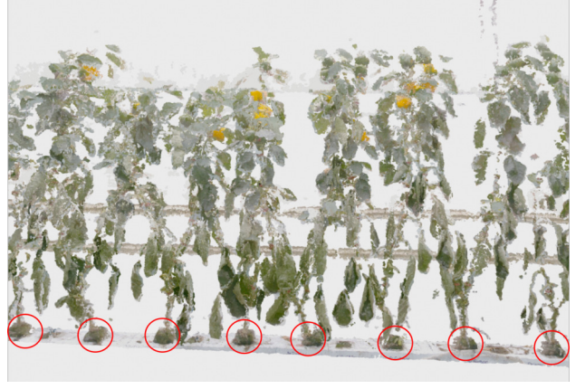
Fig. 3: An example point cloud map produced by our approach. We show in the red circles the stems of the plants that we use as temporally stable features for the registration.
