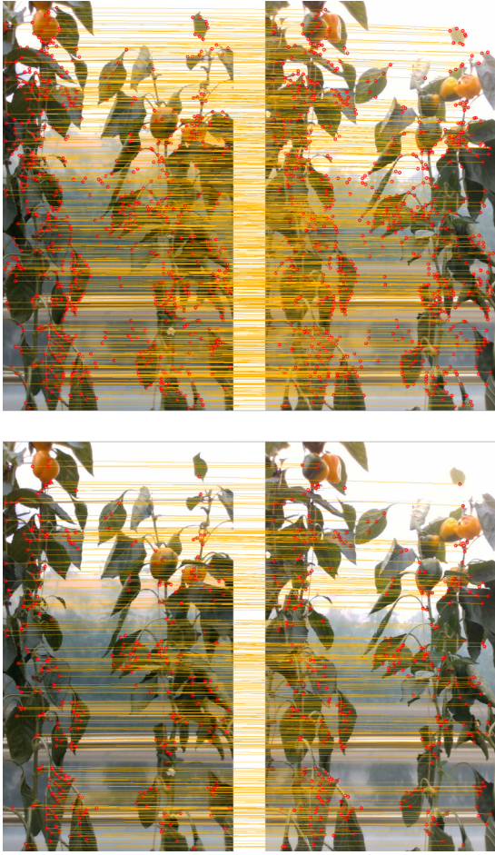
Fig. 7: On the top, the associations found by matching only SuperPoint descriptors. On the bottom, the result obtained by filtering the matches exploiting the 3D information.
