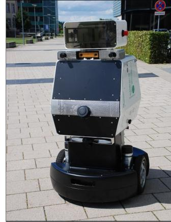
Fig. 1. The robot used within the EUROPA project offers service tasks in urban environments such as guided tours and delivery.
