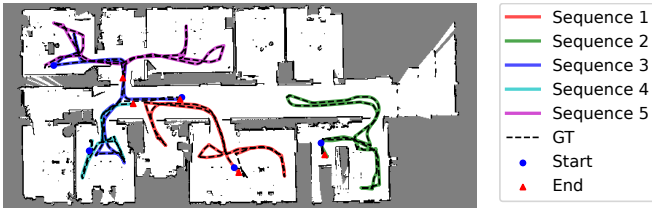
Fig. 4: Qualitative global localization results of ENM-MCL on all five sequences of the in-house dataset. We show the predicted trajectories after convergence. The predicted trajectories are mostly aligned with the ground truth, indicating the high accuracy and reliability of our method.
