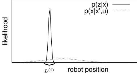
Fig. 1. The two components of the motion model. Within the interval  $L^{(i)}$  the product of both functions is dominated by the observation likelihood. Accordingly the model of the odometry error can safely be approximated by a constant value.
