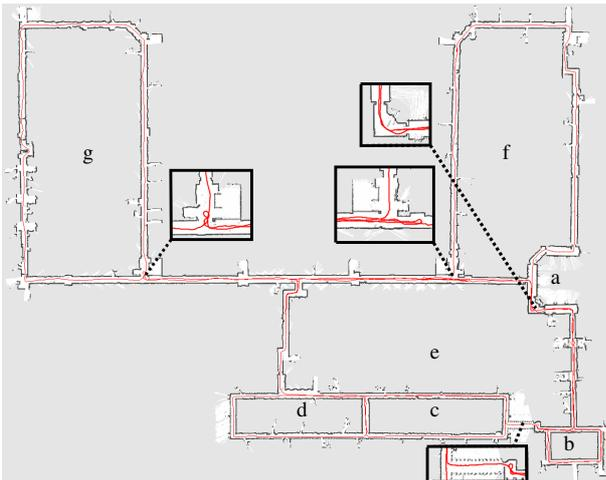
Fig. 5. **MIT Killian Court** The robot starts from the point labeled with *a*, then goes for the first loop *b*. It then moves to *c*, *d*, and comes back to *a* and *b*, prior to visit *f* and *g*. The environment is of  $250 \times 215$  m and the robot traveled for 1.9 km. This map has been generated with 80 particles. The rectangles show magnifications of several parts of the map.
