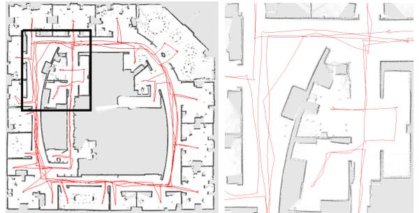
Fig. 3. **Intel Lab**, The robot starts in the upper part of the circular corridor, and runs several times around the loop, before entering the rooms. On the left, map generated with 15 particles. On the right a particular showing the accuracy of the map in the loop closure point, the resolution is 1 cm.
