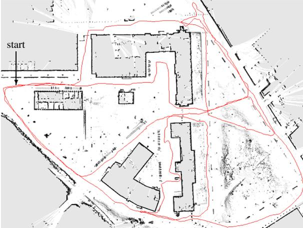
Fig. 4. **Freiburg Campus** The robot first runs on the external perimeter, for closing the outer loop. The internal parts of the campus are then visited. The area is  $250 \times 250$  m, and the overall trajectory is 1.7 km. Map generated with 30 particles.
