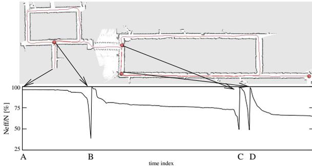
Fig. 7. The graph plots the evolution of the  $N_{eff}$  function over time during an experiment in the environment shown in the right image. The time index labeled with B corresponds to the closure of the small loop, and C, D corresponds to the big loop closure.
