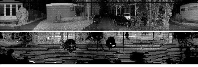
Fig. 7: Qualitative comparison between IPB Car LiDAR intensity image (up) and KITTI LiDAR intensity image (bottom) (both unprocessed). A lower vertical FoV and the uneven distribution of channels along the spinning axis makes KITTI intensity image unusable for this task.
