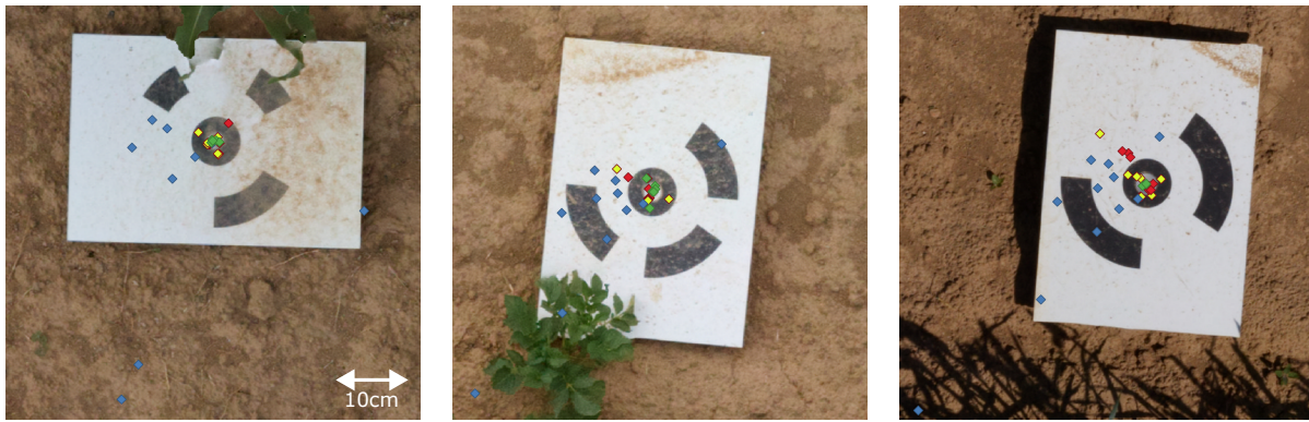
Figure 11. GCP locations of UAV1-RGB (green), UAV2-RGB (blue), UAV3-RGB (yellow), and UAV3-MS (red), for each data collection date where the GCPs are visible. The GCP locations in the orthophotos are mostly aligned across sensors and different collection dates.
