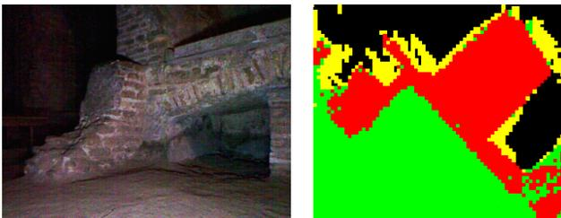
Fig. 8. A situation in which the ground level is flat and traversable but the height of the platform prevents the robot from entering the niche. Left: RGB image from the Kinect. Right: traversability estimate.
