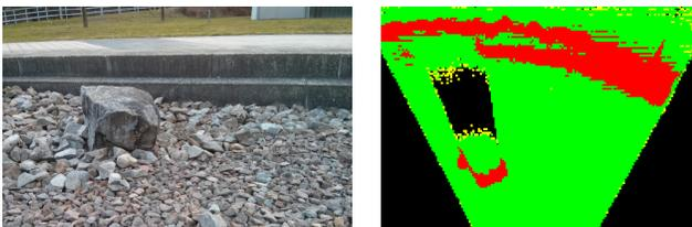
Fig. 9. Example of an outdoor scene on the Freiburg campus observed by a rough terrain robot. The left image shows a photo and the right one shows the local traversability map (distorted). The black region corresponds to the area behind the obstacle that was not visible.
