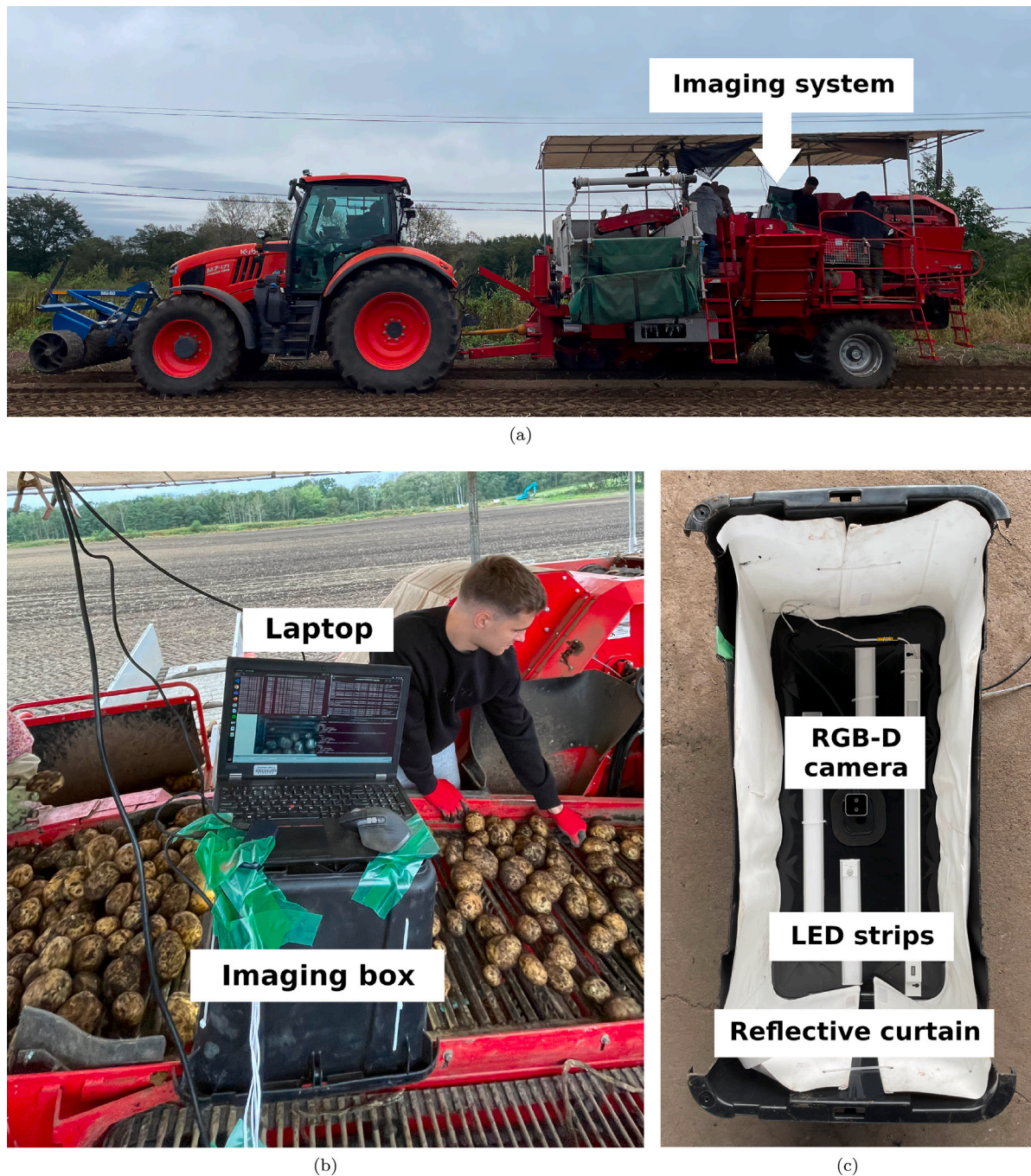
Fig. 1. (a) and (b) give overviews of the imaging system installed on a potato harvester in Sarabetsu, Japan. (c) Inside the imaging box, an RGB-D camera was installed, together with four LED strips that provided the necessary illumination inside the box. The sides of box were covered with a reflective curtain to generate diffuse lighting conditions.
