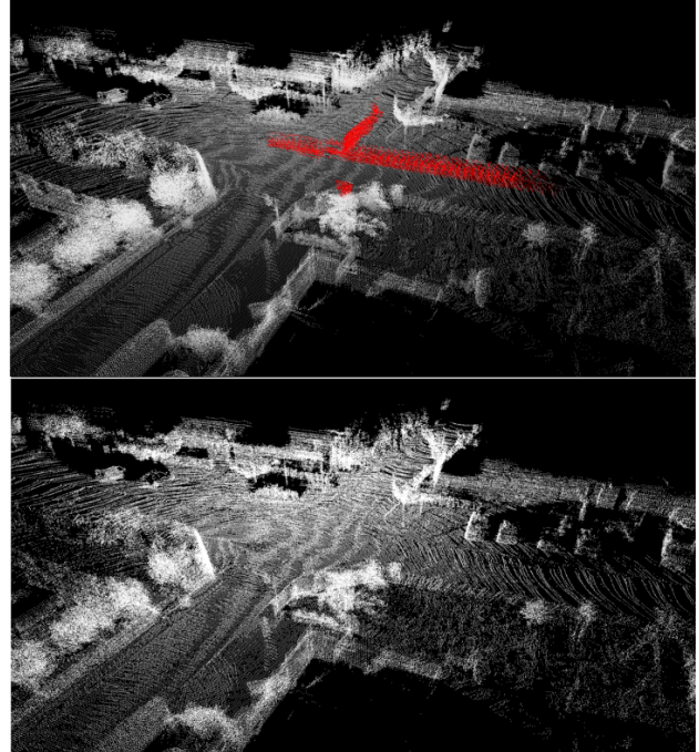
Fig. 1: The figure represents the LiDAR point cloud before (above) and after (below) applying our approach. The red points denote the dynamic and the white points the static ones. The point cloud data is from the KITTI Odometry sequence 05 frame 904 to 944.
