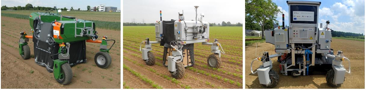
Figure 6: Different versions of the BOSCH Deepfield BoniRob used for data acquisition and deployment. Left: BoniRob V2 used for data acquisition in Stuttgart. Middle: BoniRob V3 used for data acquisition in Bonn. The acquired data is published in (Chebrolu et al., 2017). Right: BoniRob V3 equipped with the weeding module for selective spraying and stamping.
