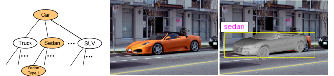
Fig. 3. Hierarchical model for object detection, including a step for determining the orientation of the object. Left : Hierarchical model with three layers. Mid : Given image. Right : Bounding box, class, and projected coarse model; from (Mottaghi et al., 2015)
