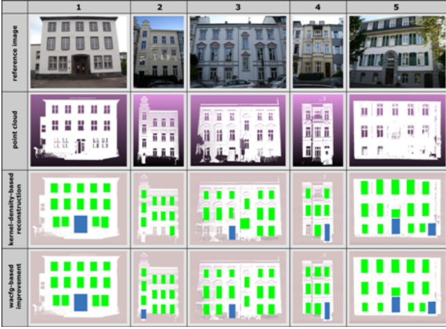
Fig. 8. Interpretation of point clouds of façades with stochastic grammars and Markov logical networks. Top row: Image of façade. Second row: Point cloud with holes. Third row: Data driven interpretation of point cloud; windows: green, doors: pink, façade: white. Last row: Model driven interpretation. Observe the predictive power of the model; from (Dehbi et al., 2016)
