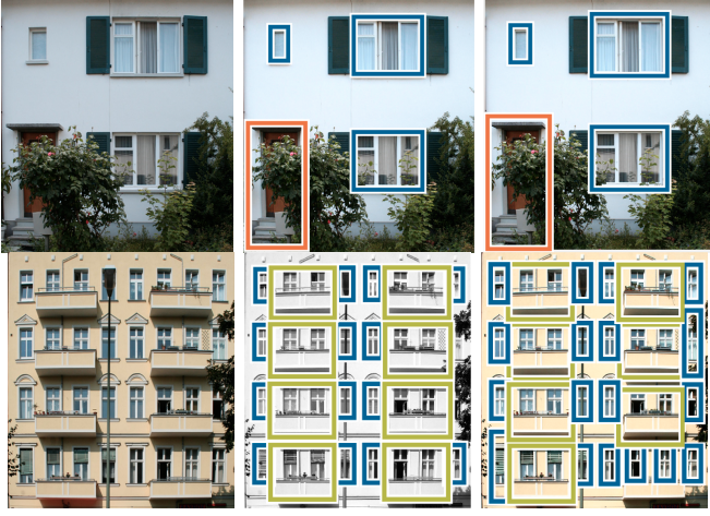
Fig. 6. Façade reconstruction based on a marked point process for façade elements (image, ground truth, reconstruction), CPU-time appr. one hour. from (Wenzel, 2016)
