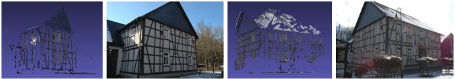
Fig. 4. Two 3D point clouds and their associated images captured at widely separated views
