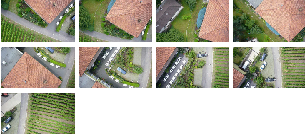
Figure 4: Every 75th of the 600 images of the real image sequence taken with the UAV at a height of approximately 30 m.
