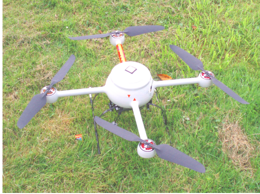
Figure 3: Used hardware. Drone MD 4-200 from Microdrones equipped with a Panasonic Lumix video camera
