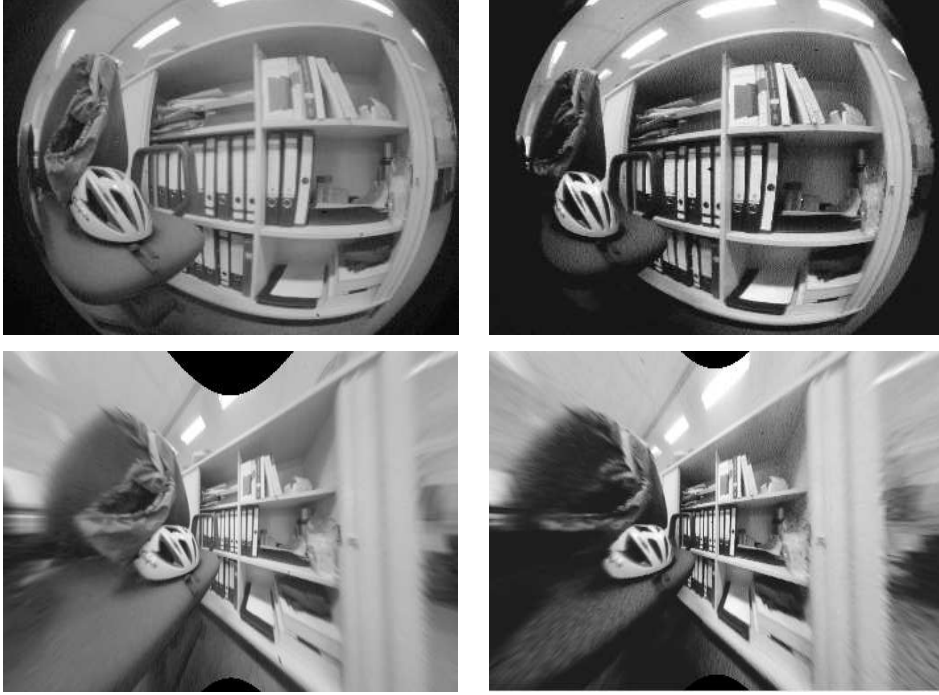
Fig. 9. Example fish-eye-stereo: Original image pair and perspective epipolar rectification
