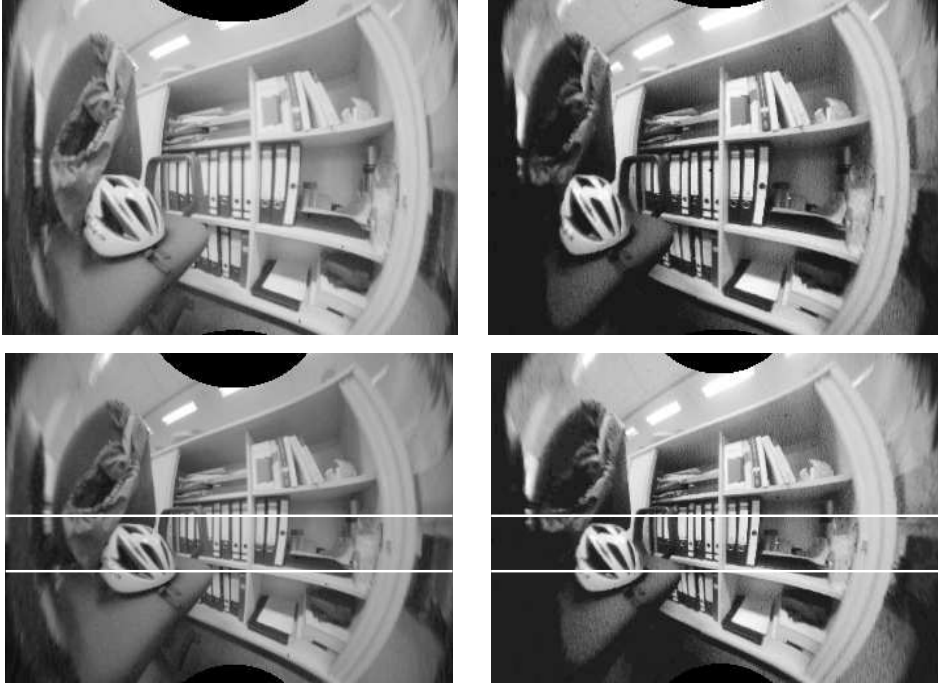
Fig. 11. Example fish-eye-stereo: Epipolar rectification with the epipolar-equi-distance ( r' = c \cdot \phi ) (top row) and the epipolar stereo-graphic r' = c \cdot \tan[0.5 \cdot \phi] rectification model (bottom row)
