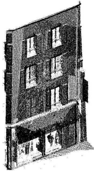
Figure 10: A facade recorded by a terrestrial laser scanner.
