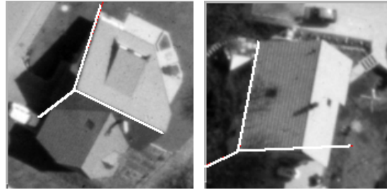
Figure 5: shows the 8 corner classes \omega_{oj}^C we are using up to now, which are sufficient for the part-of description of 4 building types, namely \{ \text{flat\_roof}, \text{non\_orthogonal\_flat\_roof}, \text{gable\_roof} \text{ and } \text{hip\_roof} \} .
