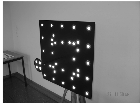
Figure 1: The used test field for calibration. The coordinates of the marks are known only approximately.
