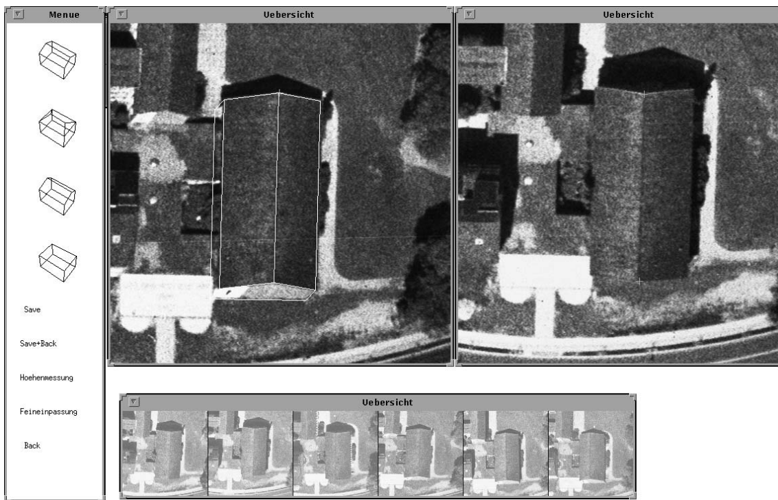
Figure 3: Semiautomatic building extraction
