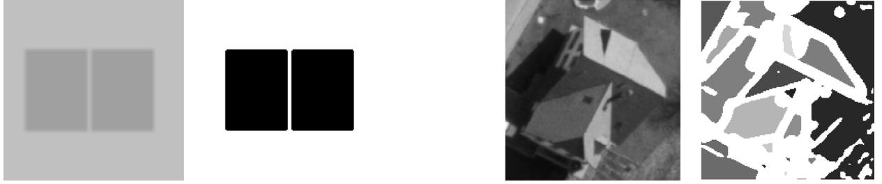
Figure 2: Examples of blob extraction. On the left blobs are extracted by thresholding, the right shows homogeneous blobs of an aerial image, labeled by grey value.
