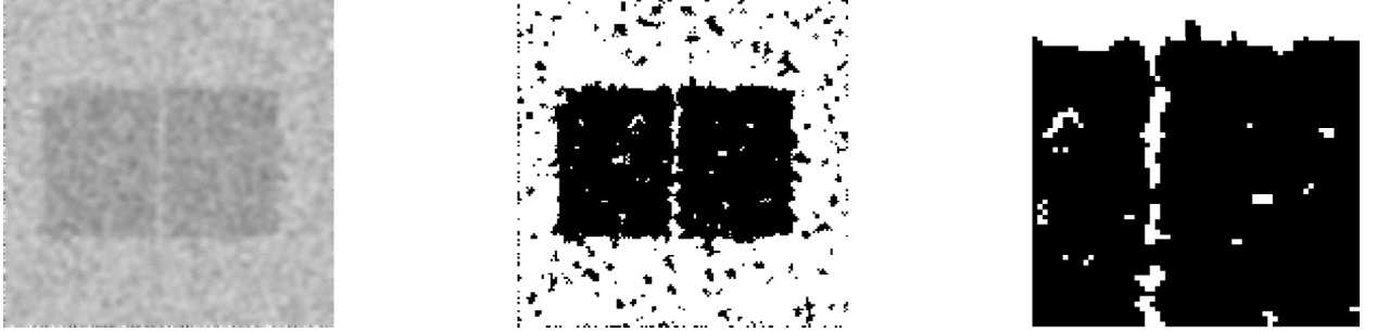
Figure 5: Artificial example of the impact of spatial uncertainty of blobs. The left shows the grey scale image from figure 2 with additional blurred Gaussian noise. The middle binary image is computed by thresholding the grey scale image. The right shows a magnified patch of the binary image.
