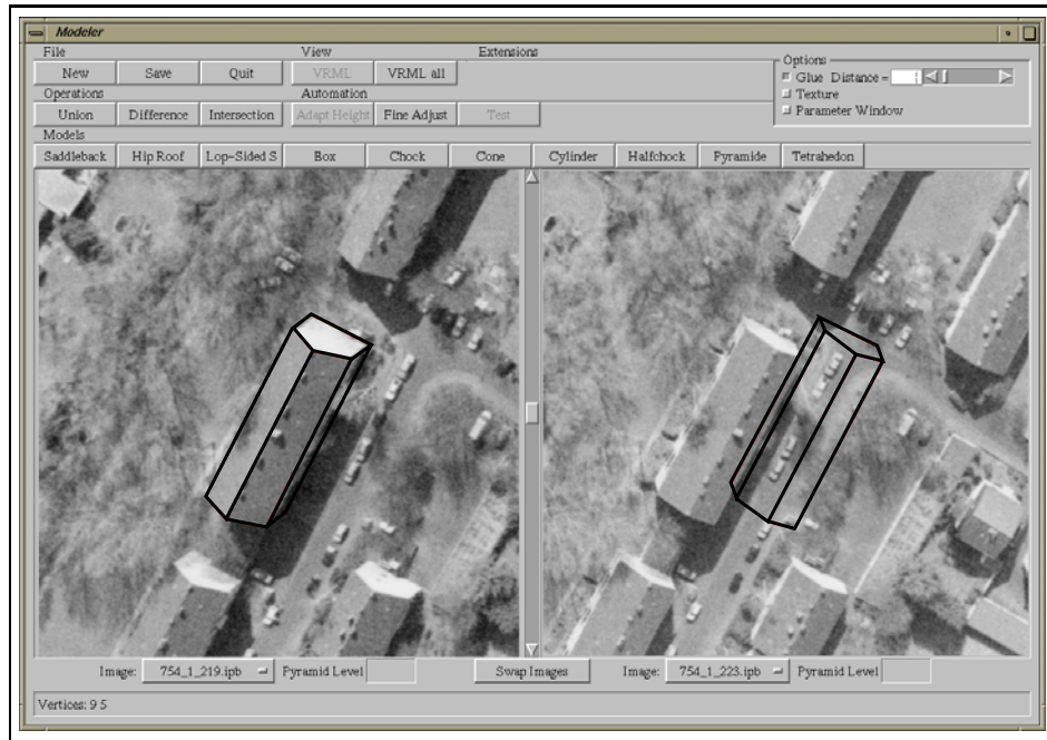
Figure 3. A 3D-primitive (saddleback-roof building) is pose and form adapted in the left image. The height is not yet measured, as shown in the right image.
