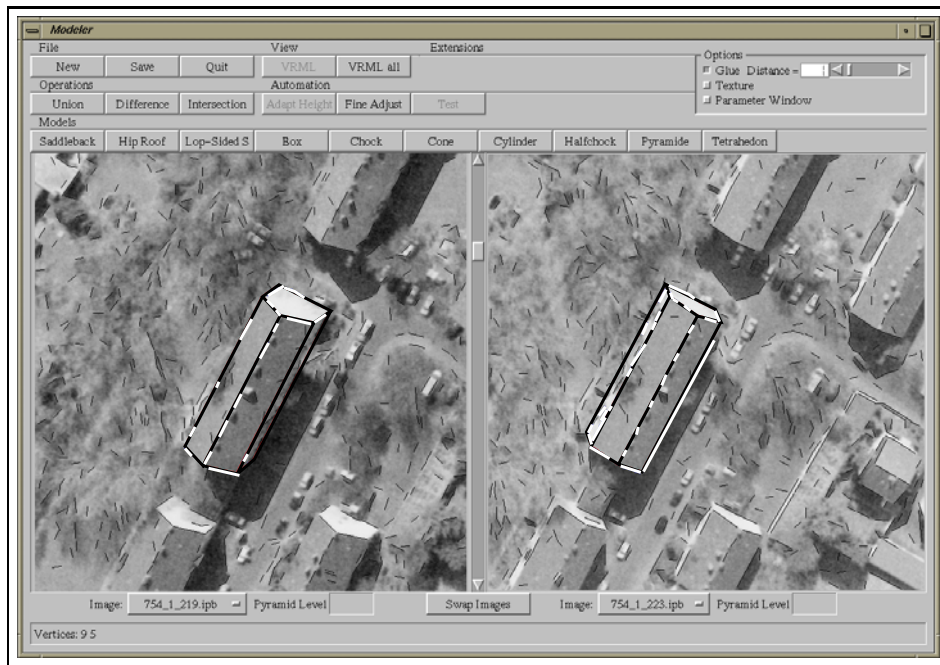
Figure 4. A 3D-primitive (thick black lines) with measured height. Some of the automatically extracted line segments (thick white lines) have been used for a final fine tuning of the parameters.
