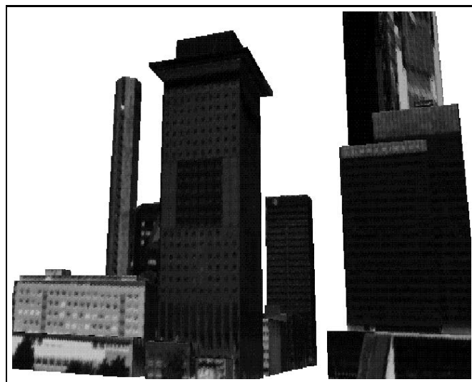
Figure 12: FRANKFURT: Automatic texture mapping and horizontal view.
