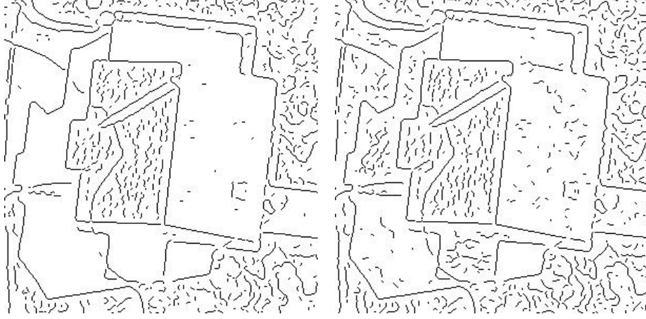
Fig. 8. shows the edges from the original image (left) and from the information preserving filtered image. Observe the low contrast edges, detected in the image filtered with IPF at the expense of getting additional, statistically significant edges, which might not be relevant.
