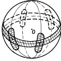
Figure 4: shows the combined distribution of all edge normals, assuming no noise, from (Wydera 1995).
