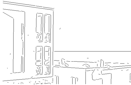
Figure 9: shows the automatically extracted edges of the nice building. Observe the few edges for the left vanishing point.
