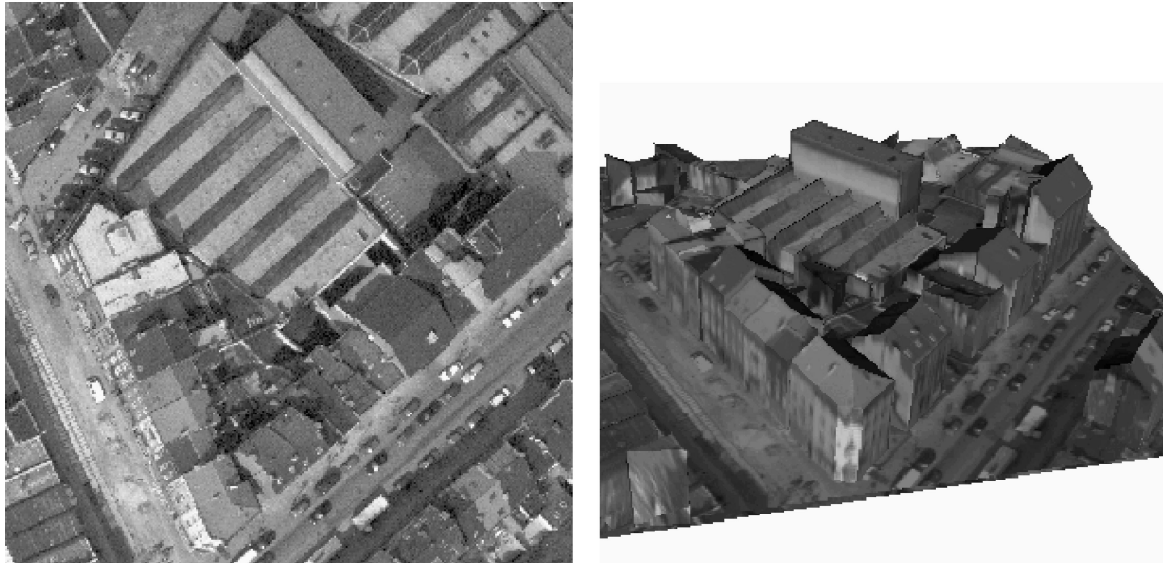
Figure 1: shows one image (section) out of 6 and the automatically derived texture mapped 3D model, from Baillard et al. 1999
