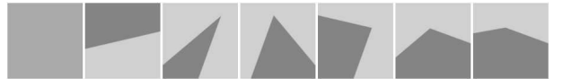
Figure 3: From left to right: a blank image, an edge with contrast \Delta g = 32 [gr], corner images with contrast \Delta g = 32 [gr] and varying angle \varphi = 30^\circ, 60^\circ, 90^\circ, 120^\circ, 150^\circ .
