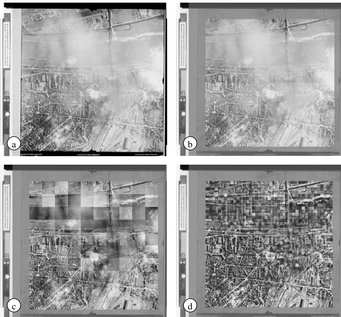
Figure 3. Dodging with histogram spreading. Part (a) shows the global approach, parts (b-d) show the results of an inner-range dodging with variable patch sizes. Therefore, we divided the image into 4 patches (b), 100 patches (c) or 400 patches (d) of equal size.
