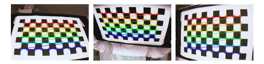
The Z coordinate of each point on the checkerboard is equal to zero
