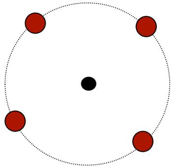
The robot can be somewhere on a circle around the landmark
