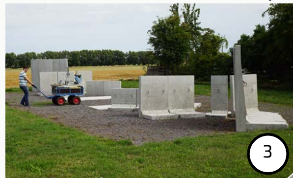
Scan with mobile scanning system
