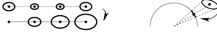
Figure 15.1: Left: Regular S -transformation of 4 2D points with full covariance matrix fixing the coordinates of the first point (translation only). Right: Uncertain homogeneous vector in \mathbb{P}^2 reduced to the uncertain 1D point on S^2
