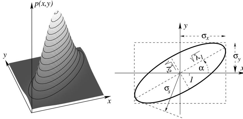
**Figure 1:** General 2D normal or Gaussian distribution, centred at the origin. **Left:** density function. **Right:** standard ellipse. Actual values:  $\mu_x = \mu_y = 0$ ,  $\sigma_x = 4.9$ ,  $\sigma_y = 3.2$ ,  $\rho = 0.7$
