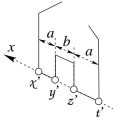
**Figure 12:** Example for the use of the invariance of the cross ratio. Due to the assumed symmetry – the distance of the door from its two neighbouring facade borders is identical to some unknown value  $a$  and the assumed knowledge about the width of the building we can infer the true width of the door in the scene from the image points
