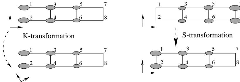
**Figure 4:** Coordinate or K-transformation and gauge or S-transformation. **Left:** K-transformation changes the reference coordinate system of the coordinates. The gauge is not changed, which here is defined by point pair (7,8). **Right:** S-transformations change the gauge of a covariance matrix, here from point pair (1,2) to point pair (7,8). The coordinates are not changed
