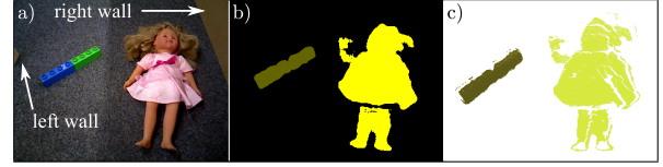
Fig. 6. Data processing for the RGBD data. a) The original RGB image containing a doll and toy blocks between two walls. b) Semantic segmentation results using the Bonnet framework [7]. c) Segmented point cloud of the corresponding objects, using the depth image to get the spatial information of each marked pixel.
