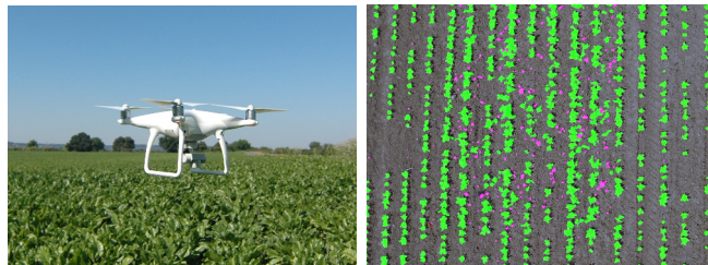
Fig. 1: Low-cost UAV used for field monitoring (left) as well as an example image analyzed by our approach (right).
