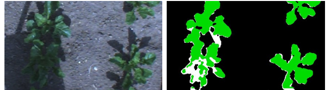
Fig. 8: Left: Detailed view on RGB image containing sugar beets. Right: Masking based on NDVI (white) and ExG (green). All vegetation pixels detected by ExG based approach are also detected by the NDVI based approach
