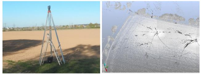
**Figure 10.** Left: special extra-high tripod equipped with a FARO X130 terrestrial laser scanner. Right: part of the registered point cloud of the sugar beet field. The black lines show false measurements.
