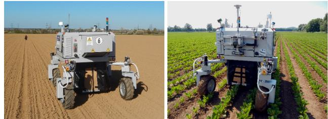
**Figure 1.** Field robot BoniRob operating on the field. Left: data acquisition three days after plant emergence. Right: data acquisition five weeks after emergence.
