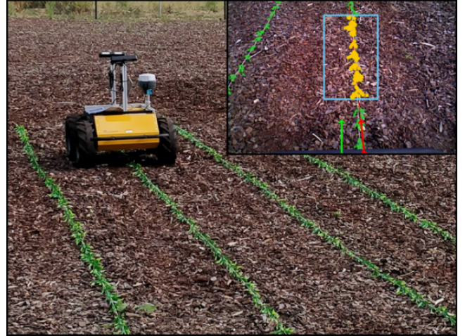
Fig. 1: Robot navigation in a test row-crop field. Top-right: on-board camera image. The visual servoing based controller executes the velocity control that brings the crop row (red arrow) to the center of the camera image (green arrow). The blue box shows the sliding window used for tracking the row along which the robot navigates.
