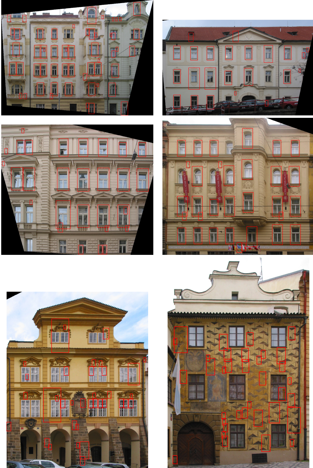
Figure 6: Examples of the T-style window detector output on images from the test set. The bottom row show the result when there are no T-style windows in the facade. Average confidence value for the images (left to right, top to bottom), T-style windows present: 16.4, 14.9, 16.4, 15.7, no T-style windows: 12.6, 14.1. Note that the radial distortion is not removed from the left image in the middle row and still good results are obtained.
