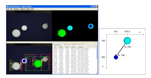
Fig. 4. Left: Intermediate scene interpretation as an instance of lay-dinner-for-two. Objects in natural colours are supported by evidence, objects in artificial colours are hypotheses based on high-level conceptual knowledge. Hypotheses are shown at the center of boxes, which represent possible locations. The low-level result is presented at top right; the original video at top left. Right: Hypothesized approach object for cup and saucer.
