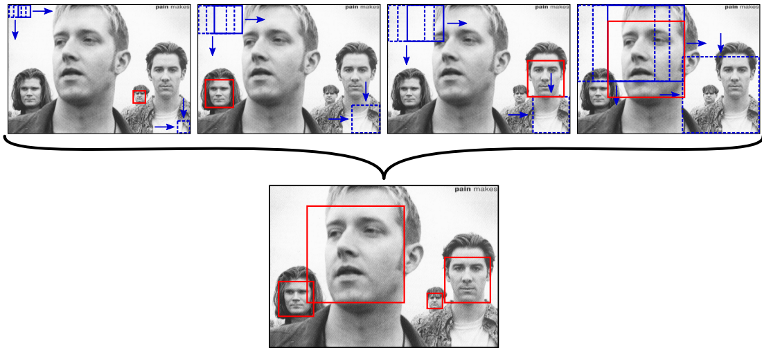
Figure 6.1: The scanning window approach to face detection. A detection window is swept through the image and an object vs. background classifier is evaluated at each position and scale.
