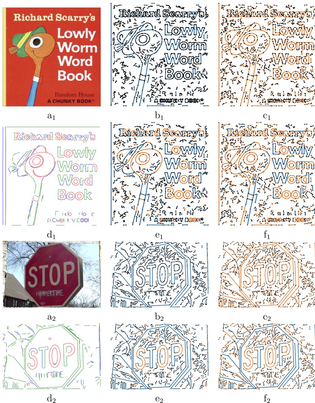
Figure 3: Pre-segmentation circlePeucker vs. Douglas-Peucker (Best viewed in colour). a<sub>\*</sub>: Given images as used in (Patraucean et al., 2012). b<sub>\*</sub>: Pre-Segmentation using Douglas-Peucker. c<sub>\*</sub>: Pre-Segmentation using circlePeucker. e<sub>\*</sub> and f<sub>\*</sub>: Final segmentation using b<sub>\*</sub> and c<sub>\*</sub>, respectively. d<sub>\*</sub> results by ELSD. Colours, see Fig. 1 and 2.
